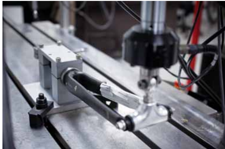
A carbon road fork undergoing ultimate strength testing
